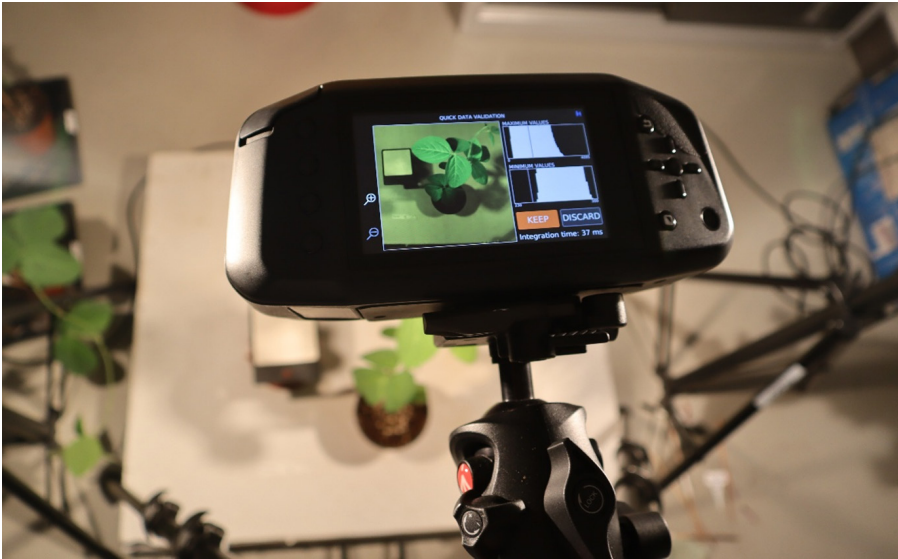
Figure 2. Using hyperspectral camera to capture leaf area
