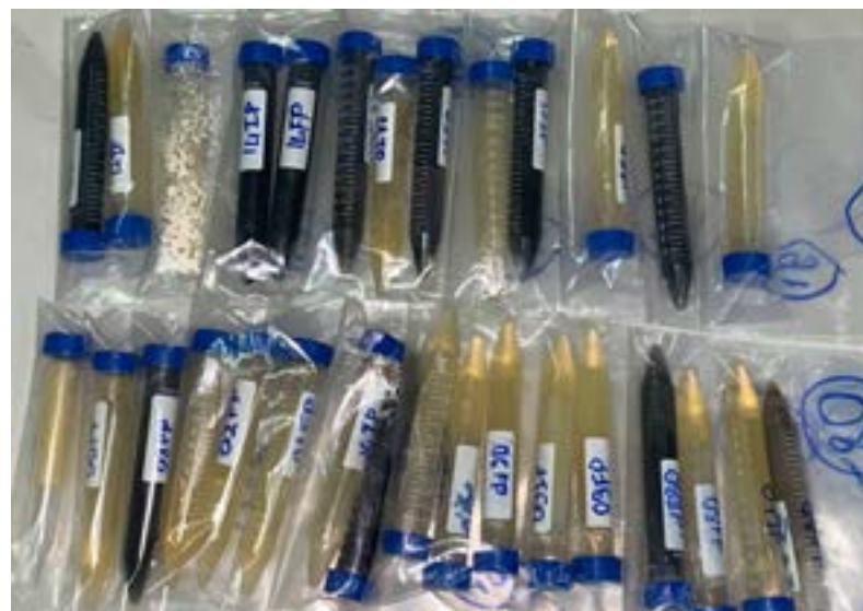
Figure 4. E. coli test result in drinking water after incubate in dark room for 3 days (room temperature)
